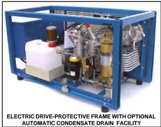
The electric models use a standard Molecular Sieve/ Activated Charcoal/Molecular Sieve format, whilst the Petrol and Diesel driven unit have an additional layer of Hopcalite catalyst to convert any traces of Carbon Monoxide to relatively harmless Carbon Dioxide.
