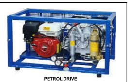
The electric models use a standard molecular sieve/ activated charcoal/molecular sieve format, whilst compressors driven by petrol or diesel engines have an additional layer of Hopcalite catalyst to convert any traces of carbon monoxide from the engine exhaust fumes to relatively harmless carbon dioxide.
