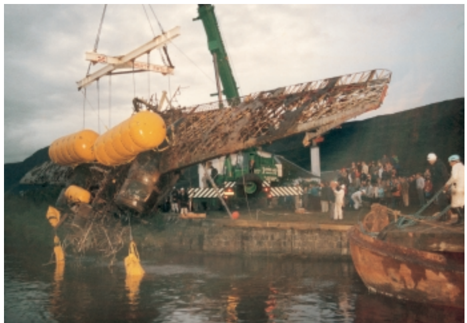
Submerged crash sites perhaps offer the best potential for the future. The remains of a Wellington bomber which crash-landed in Loch Ness on New Year's Eve 1939 are seen here being recovered in 1985. Carefully restored, the aircraft is now displayed at Brooklands Museum and is one of only two complete Wellingtons known to survive out of a total production run of 11,500. (Photograph by kind permission of Brooklands Museum)
