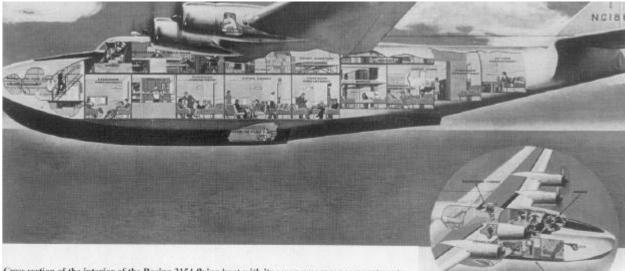
Cross section of the interior of the Boeing 3154 flying boat with its seven passenger compartments, including the deluxe suite in the tail.
